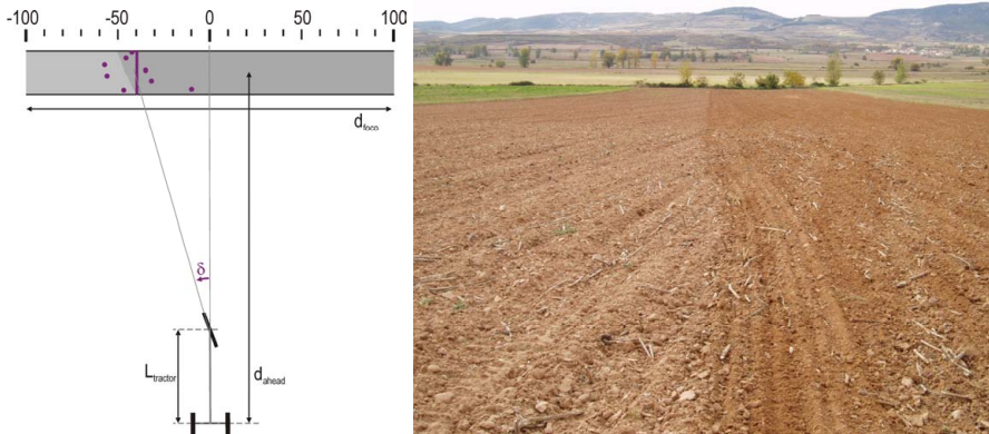
Fig. 9. Left: Graphic representation of the control law. Right: The dark area corresponds with the cultivated area by means of artificial vision. The light area is the non-cultivated area.
